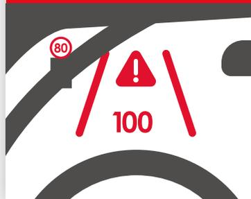
The diagram shows a driver's perspective from the dashboard. A speedometer displays a red limit line at 100 km/h. A red exclamation mark icon is shown above the speedometer, indicating a warning when the current speed exceeds the recommended limit for the road conditions.
